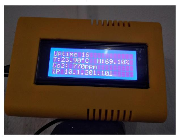
The rigged setup now runs over 1,5 years under roughest conditions and still works perfect, which really is remarkable for a gas sensor thanks to the robust design of the S8.
